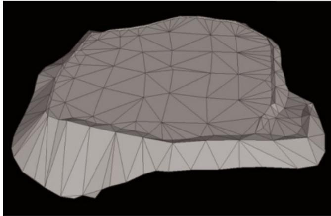
Figure 4: GNSS RTK surveyed 220 point mesh of 372 faces.
