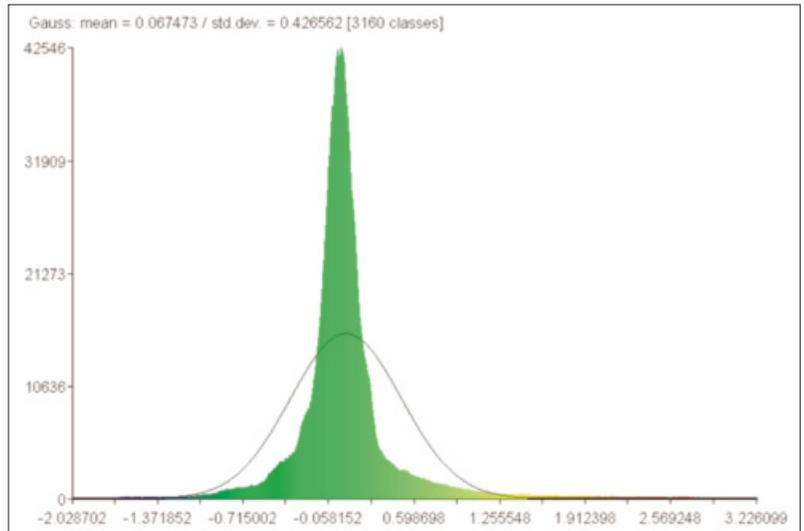
Figure 9: C2M distances—UAV DSM point cloud vs. GNSS mesh.
