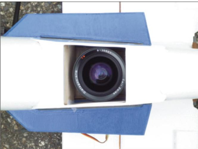
Figure 3: UAV payload—Samsung NX1000 with Carl Zeiss 18mm lens.
