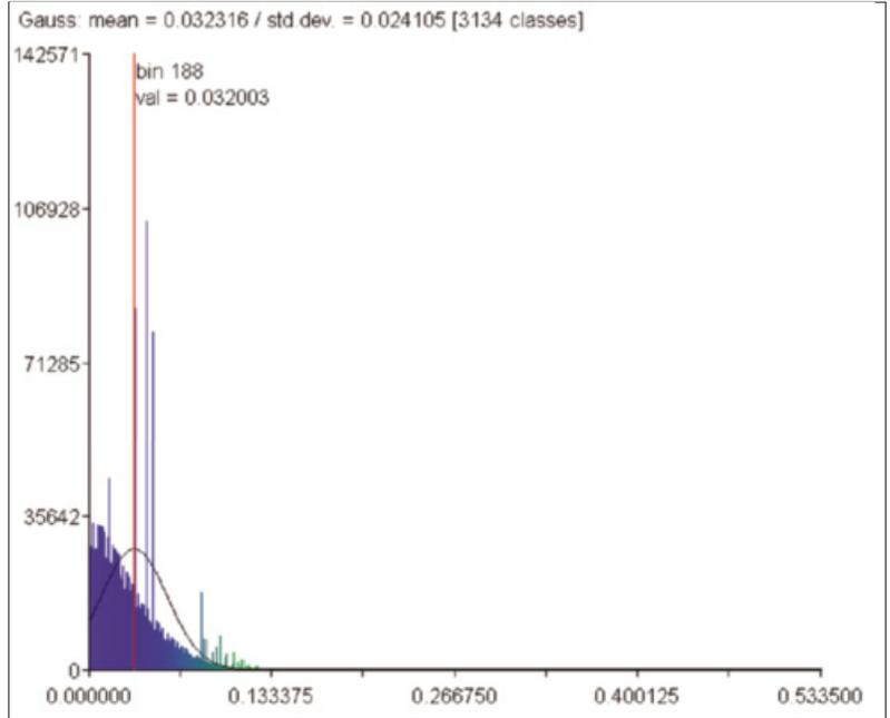
Figure 11: Cloud to cloud absolute distances for 9.8 million distances between flight 1 and 2 surfaces.
