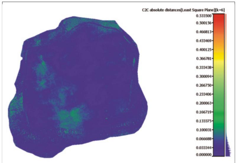
Figure 12: Cloud to cloud absolute distances between flight 1 and 2 surfaces.
