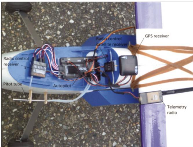
Figure 2: UAV autopilot, sensor, and radio packages.
