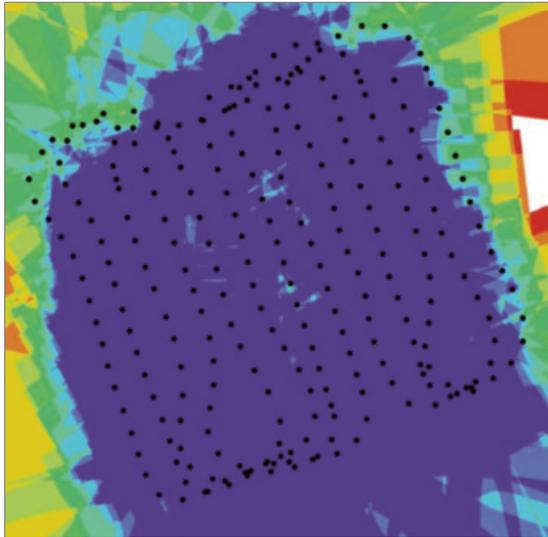
Figure 7: Flight lines with photo locations.
