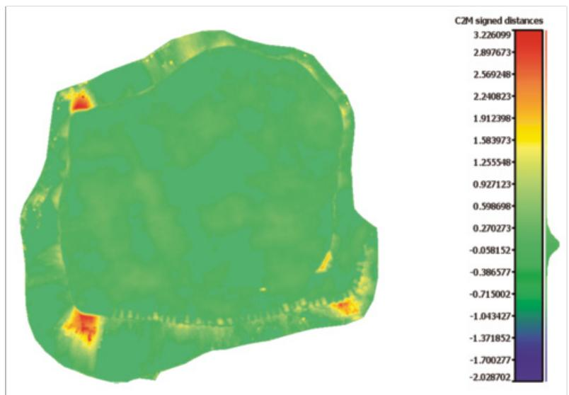
Figure 10: C2M signed distances—UAV DSM vs. GNSS survey.
